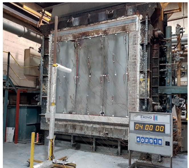
Third party, bi-directional fire testing to ensure fire integrity
