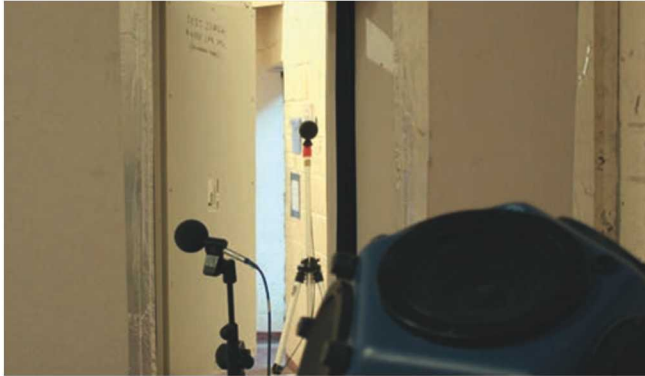
Profab access panel undergoing acoustic testing
